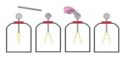
The electroscope keeps being neutral, but the closest area to the positive rod has an excess of electrons and the area which is further has a lack of electrons. The closest area to the negative rod has a lack of electrons and the furthest area has an excess. You can charge the electroscope as it is shown in the pictures.
