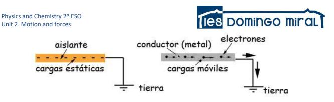
Examples of isolator materials are wood, plastics, glass and rubber. Metals are conductors and some dissolutions too (for example, salt dissolved in water).
