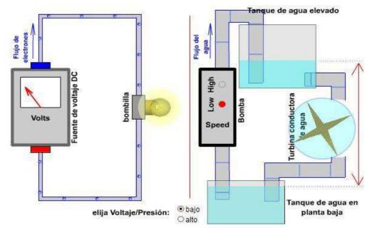
Now, look at the electric circuit. It is easy to identify the equivalent to the flow: the intensity of the current. Just as like water, that needs a pump that impulses it to continue its flow, charges need a booster that allows it to continue flowing. This device is called a generator.
