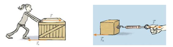
As you know, it is different to drag the wooden block by different surfaces: frictional force depends on the nature of the surfaces in contact. The rougher they are, the greater the friction force will be and the more polished the surfaces are, the frictional force will be smaller. This is why walking on ice is more difficult than on asphalt, as the frictional force is much lower.
