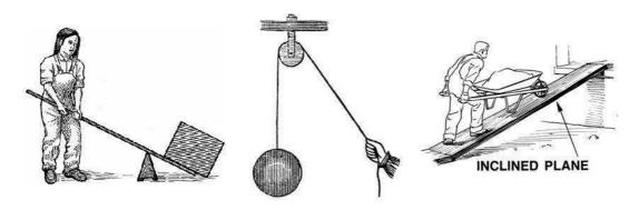
Some of the simplest machines are the lever, the pulley and the inclined plane. Let's study them.
